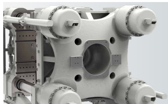
The four short-stroke clamping cylinders on the fixed platen ensure a fast and uniform clamping force with real-time monitoring by a pressure sensor and high repeatability.
